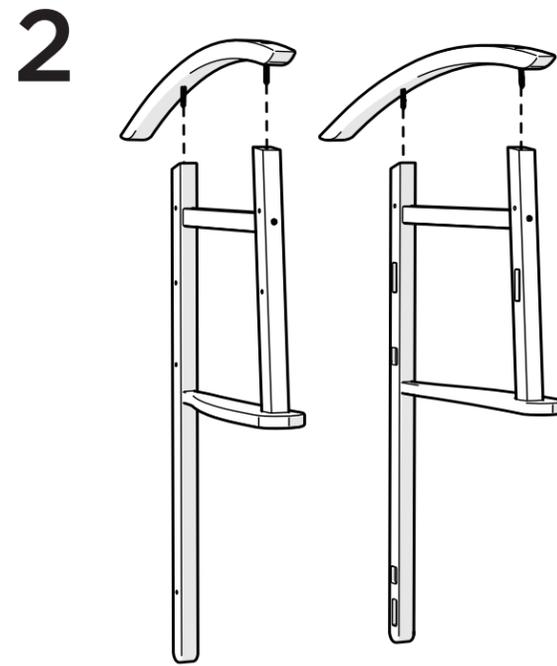
Partially thread each screw into pilot holes by hand before fully tightening.
