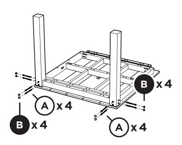
NOTE - Ensure thru holes in legs line up with pilot holes in aprons.
