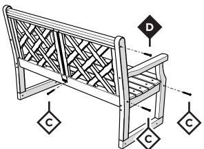
Assembly tip for step 5: Prop up one side of the bench at least 2.5" for ease of assembly
