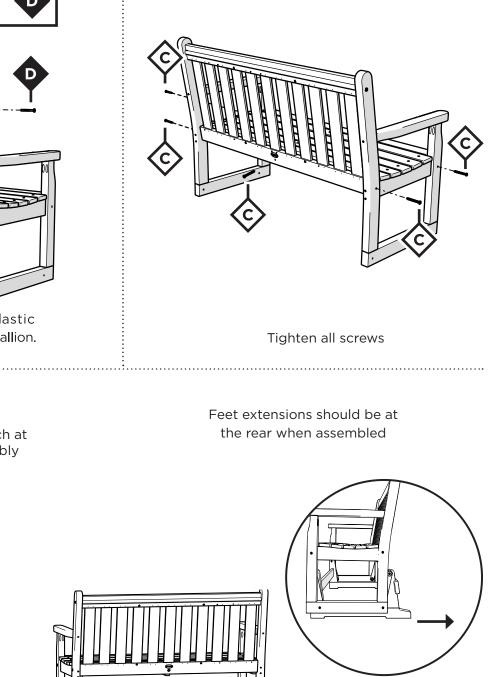
Installing the base backwards could result in the glider tipping over unexpectedly
