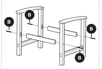
Do not tighten screws until last step
