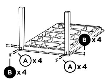
NOTE - Ensure thru holes in legs line up with pilot holes in aprons.
