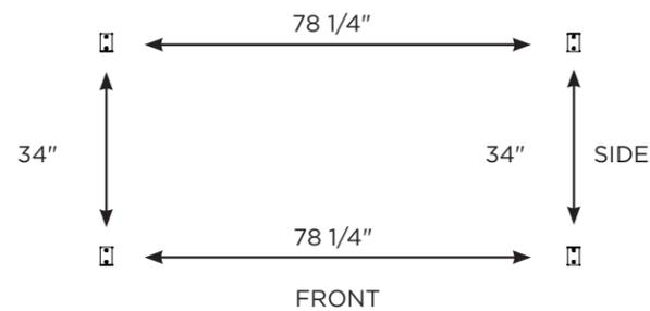
**NOTE:** Dimensions of the hanging brackets are to the center of the brackets.
