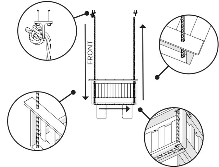
Continue pulling the rope through the arm until the knotted end is stopped by the front overhead hanging brackets.
