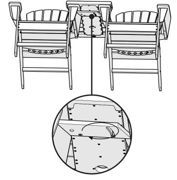
To lock in place, rotate SLIDE Lock forward.
