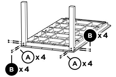
NOTE - Ensure thru holes in legs line up with pilot holes in aprons.
