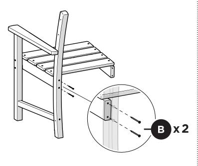
Allign screws with predrilled holes in the seat assembly.
