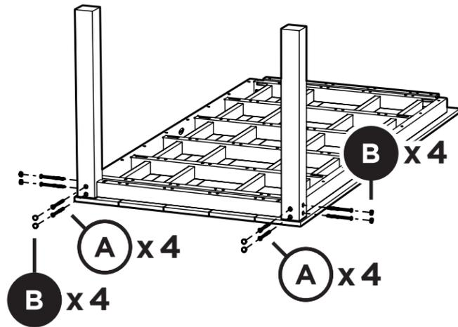
NOTE - Ensure thru holes in legs line up with pilot holes in aprons.
